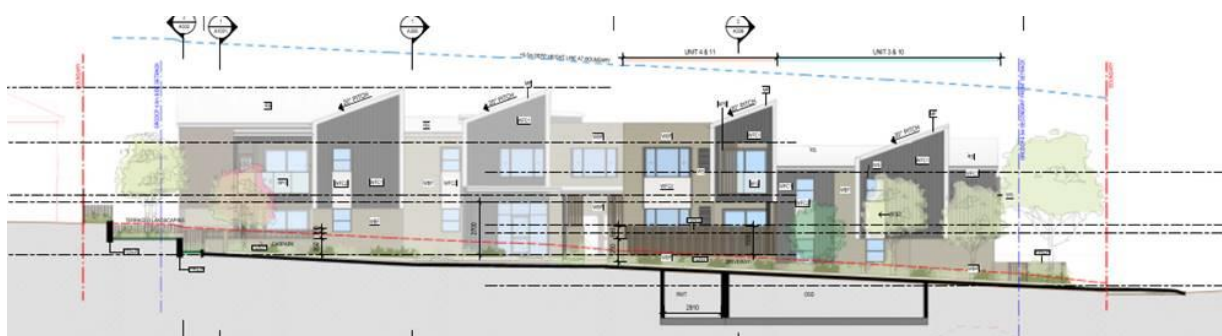
Figure 02 – Proposed excavation to accommodate rainwater tank and OSD
